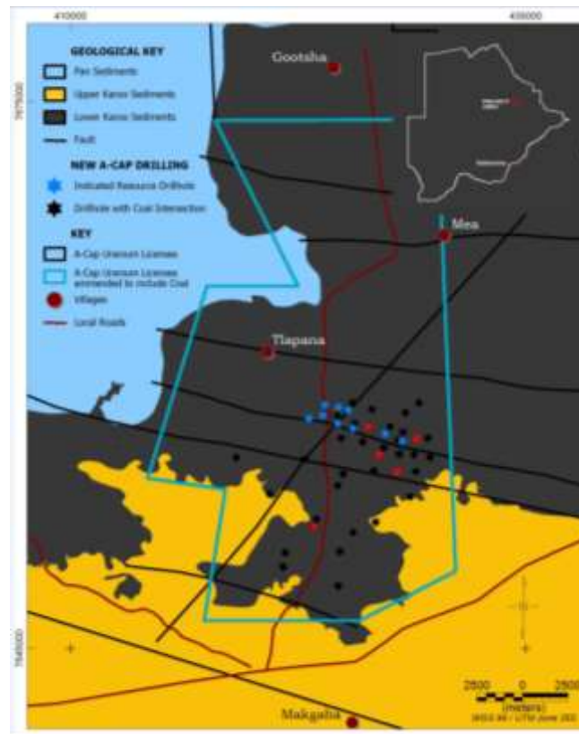
Figure 5: Plan view of the Mea Coal Project showing the location of all drill holes to date. Black stars are percussion holes, red stars are diamond core holes.
