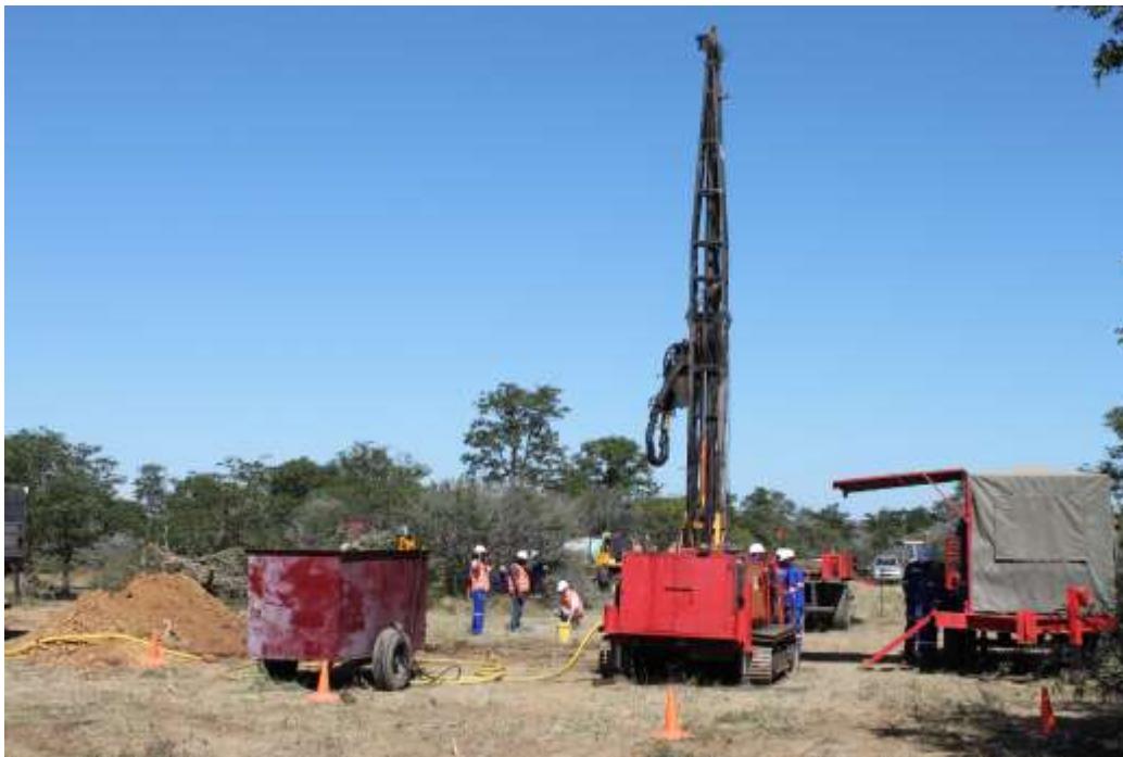
Figure 1 Diamond drilling currently underway
